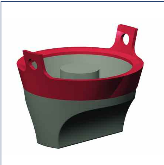
3-D model of conductive silicone custom masking for appliance knob allows part to be masked and hung from integrated tabs.
