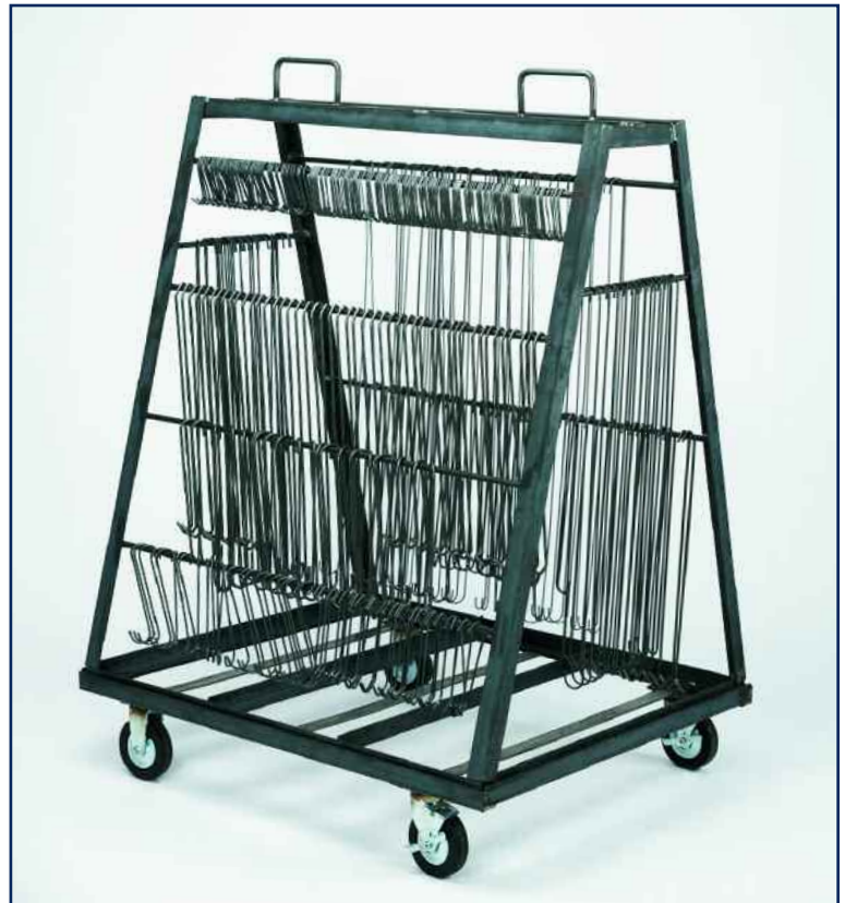
Integrated hook storage and burn-off cart. Top frame lifts off base and placed directly on burn-off trolley.
